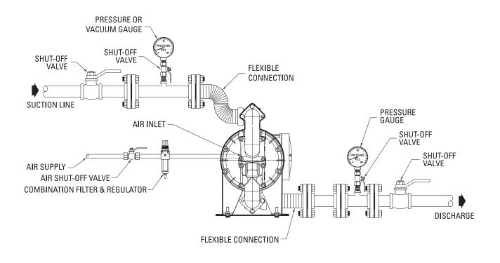
**NOTE**: In the event of a power failure, the shut-off valve should be closed, if restarting of the pump is not desirable once power is regained.
