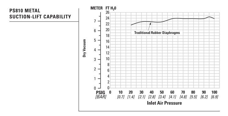
Suction-lift curves are calibrated for pumps operating at 305 m (1,000') above sea level. This chart is meant to be a guide only. There are many variables that can affect your pump's operating characteristics. The number of intake and discharge elbows, viscosity of pumping fluid, elevation (atmospheric pressure) and pipe friction loss all affect the amount of suction lift your pump will attain.
